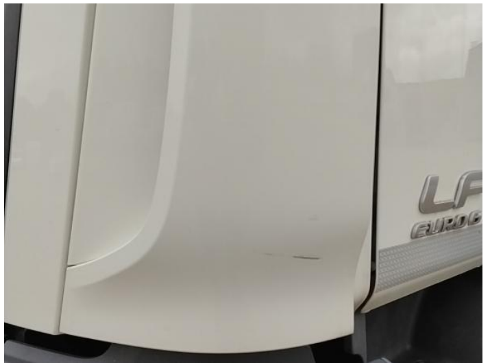
6: Wing nsf Scratched UpTo 25mm Thru Paint
