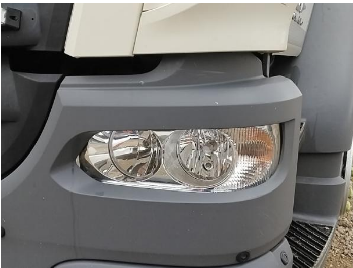
5: Fog Lamp Surround nsf Scuffed (Unpainted) UpTo 100mm
