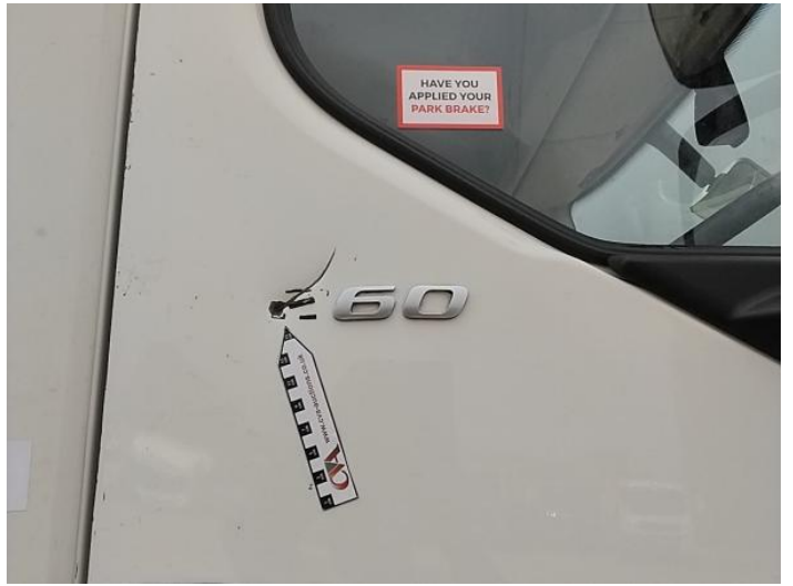
12: Door osf Dented With Paint Damage
