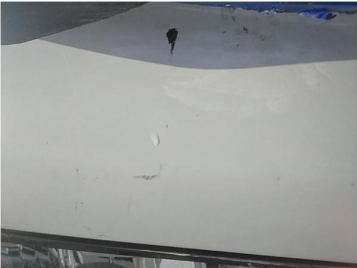
1: Bumper Front Scratched UpTo 25mm Thru Paint
